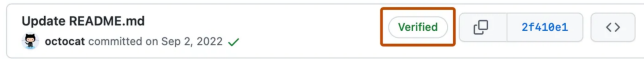
Fig. 6. An Example of a verified commit: Once a GitHub user enables commit signing and uses 'git commit -S -m,' their commits will be marked as verified.
